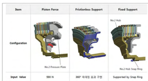
Clutch Pack Structural Analysis
